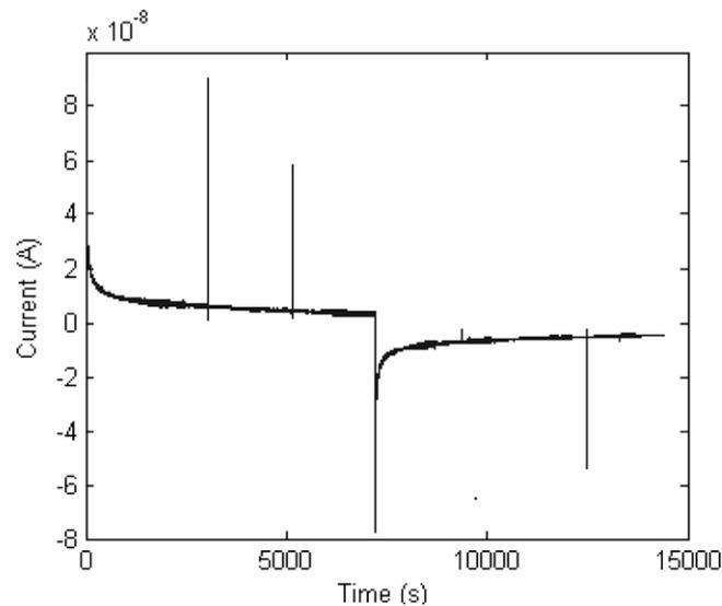
Fig. 1. Real-life noisy PDC waveform.
