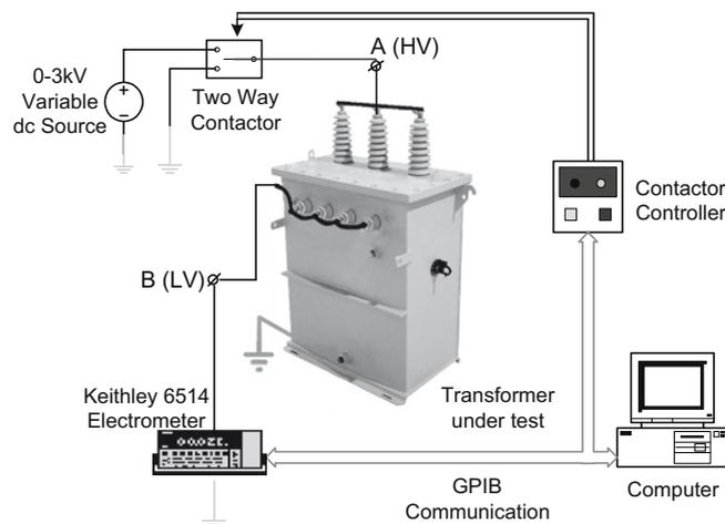
Fig. 5. Schematic diagram of experimental setup.
