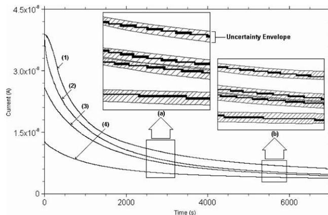
Fig. 17. Denoised version of four polarization curves.
