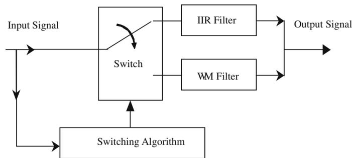
Fig. 2. Schematic representation of the hybrid filter.
