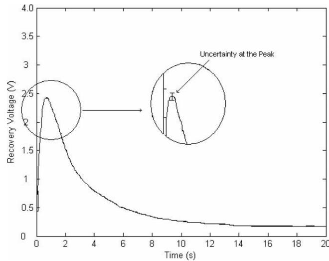
Fig. 15. Recovery Voltage waveform denoised with hybrid filter.
