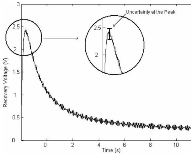
Fig. 13. Real-life noisy Recovery Voltage waveform.
