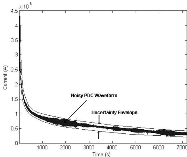
Fig. 10. Uncertainty envelope of noisy data, acquired during polarization current measurement.
