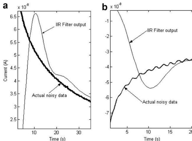
Fig. 4. Real-time noisy recorded data and lowpass IIR filter output in the initial stage of: (a) polarization current and (b) depolarization current.
