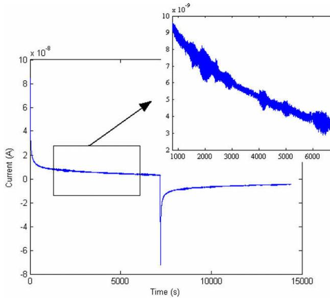
Fig. 3. WM filter output of a real-time noisy PDC waveform.
